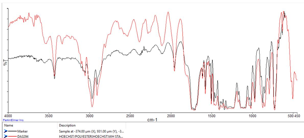
**Figure 5-1. FT-IR spectra of analysed PET powder (black line) and reference FT-IR spectra of PET-polymer from the library (red line) (match score of 0.98 in transmission mode)**
