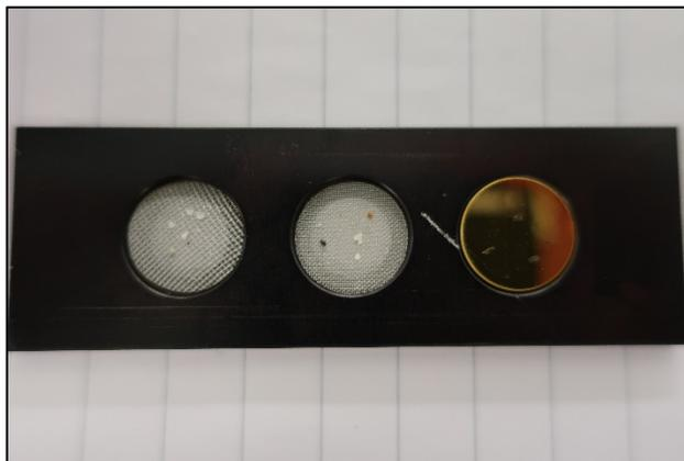
**Figure 3-7. Picture of random selection of particles from a sample (VI03) placed on steel mesh filters and a gold plate for FT-IR analysis.**
