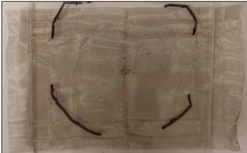
**Figure 3-5. Photo of processed sediment sample, collected on a 45  $\mu\text{m}$  steel mesh and placed between two acryl plates for visual microscopy.**
