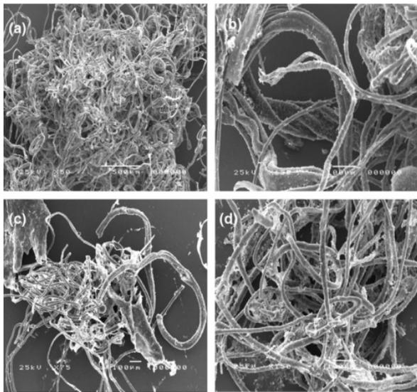
**Figure 5.** Scanning electron microscope (SEM) pictures of plastics found in *Nephrops norvegicus* (Clyde Bay, Scotland). Picture taken from Murray et al. 2011<sup>93</sup>.
