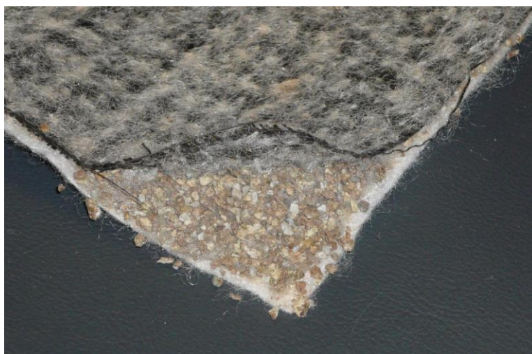
Figur 5: Bentonittleire (granulat) i fiberduk. Foto: www.claysandminerals.com .
