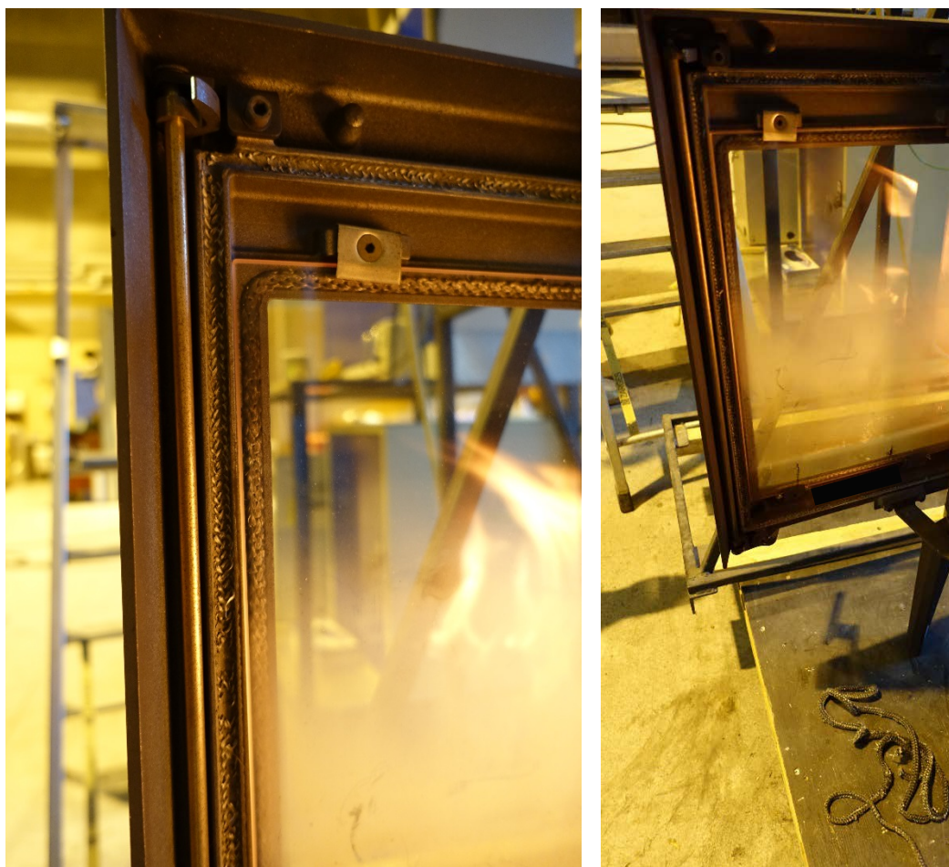
Figure 9: Woodstove door after removal of the gasket.
