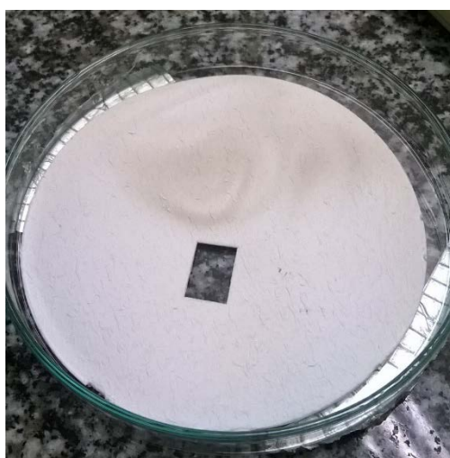
Figure 17: Example of sample for EC/OC analysis taken from one quartz filter with a trace of leakage.
