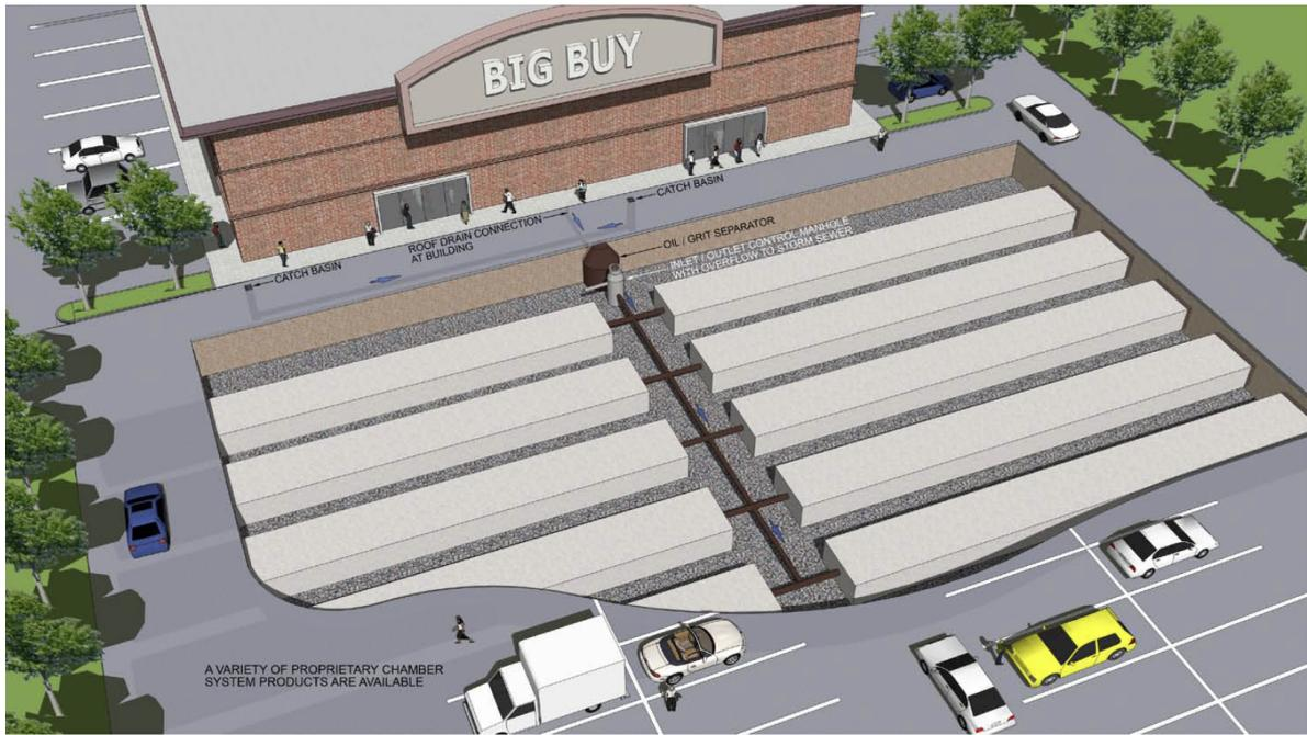
**Figure 6.12** Schematic design of an **infiltration chamber system** below a parking lot (CVC and TRCA 2010)
