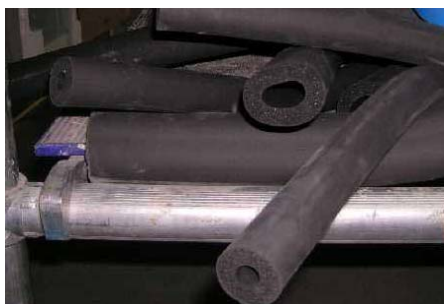
Cellular rubber used for insulation of tubing, and plastics in electronic equipment may contain brominated flame retardants. Photo: SFT
