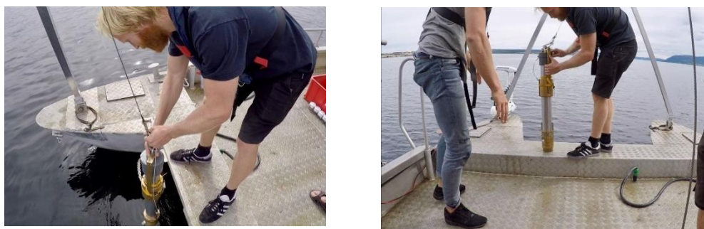
Figure 2. Deployment of Kajak-Brinkhurst sediment corer during sampling in Lake Mjøsa and Lake Femunden. Images show core being deployed (A) and retrieved (B) at the stern of the vessel. Images: David P. Eidsvoll, NIVA.
