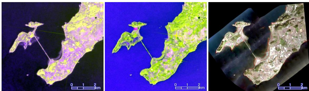
Figure 22. (Left) Minimum and (middle) maximum Sentinel-1 backscatter mosaics and (right) the detected intertidal zone area (red line) superimposed on an aerial image over Tautra.
