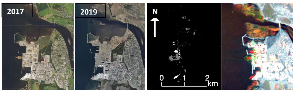
Figure 33. Detected changes in the harbour of Verdal from 2017 to 2018 by thresholding the difference of the 95% percentile images from both years. The aerial images date from 30 June 2017 and 17 May 2019.
