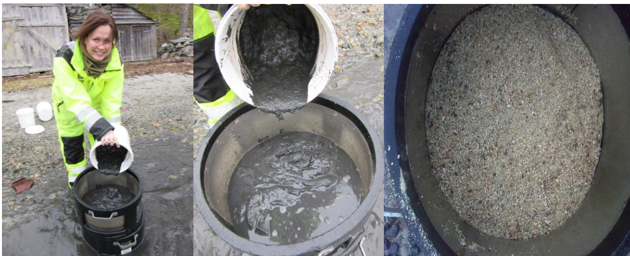
Figure 6. Sieving of sediment samples. Sediment collected from directly under the fish farm was dark grey, and smelled of H_2S (photos: Sigurd Øxnevad, NIVA).
