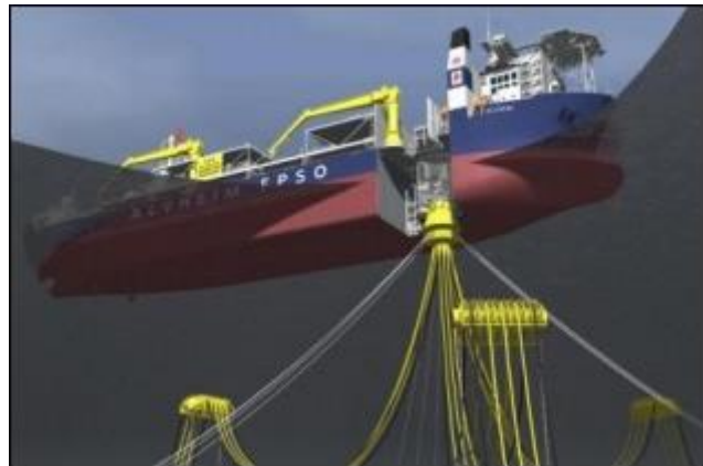
Figure 7 Alvheim FPSO. Sketch of the turret configuration (Source: Oljefakta.no)
