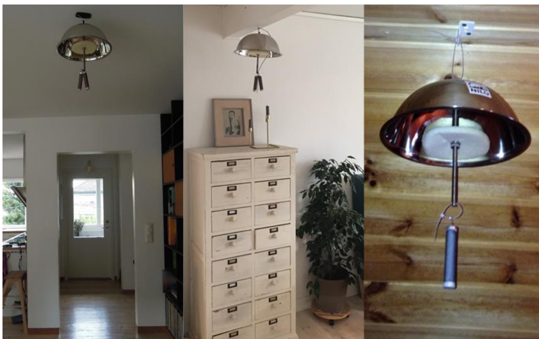
Figure 1: Air sampling equipment: PUF-PAS (top) and XAD-PAS (bottom), used to perform screening in indoor residential environments.
