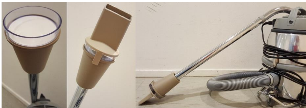
Figure 2: Sampling equipment for sampling of floor dust in indoor residential environments.
