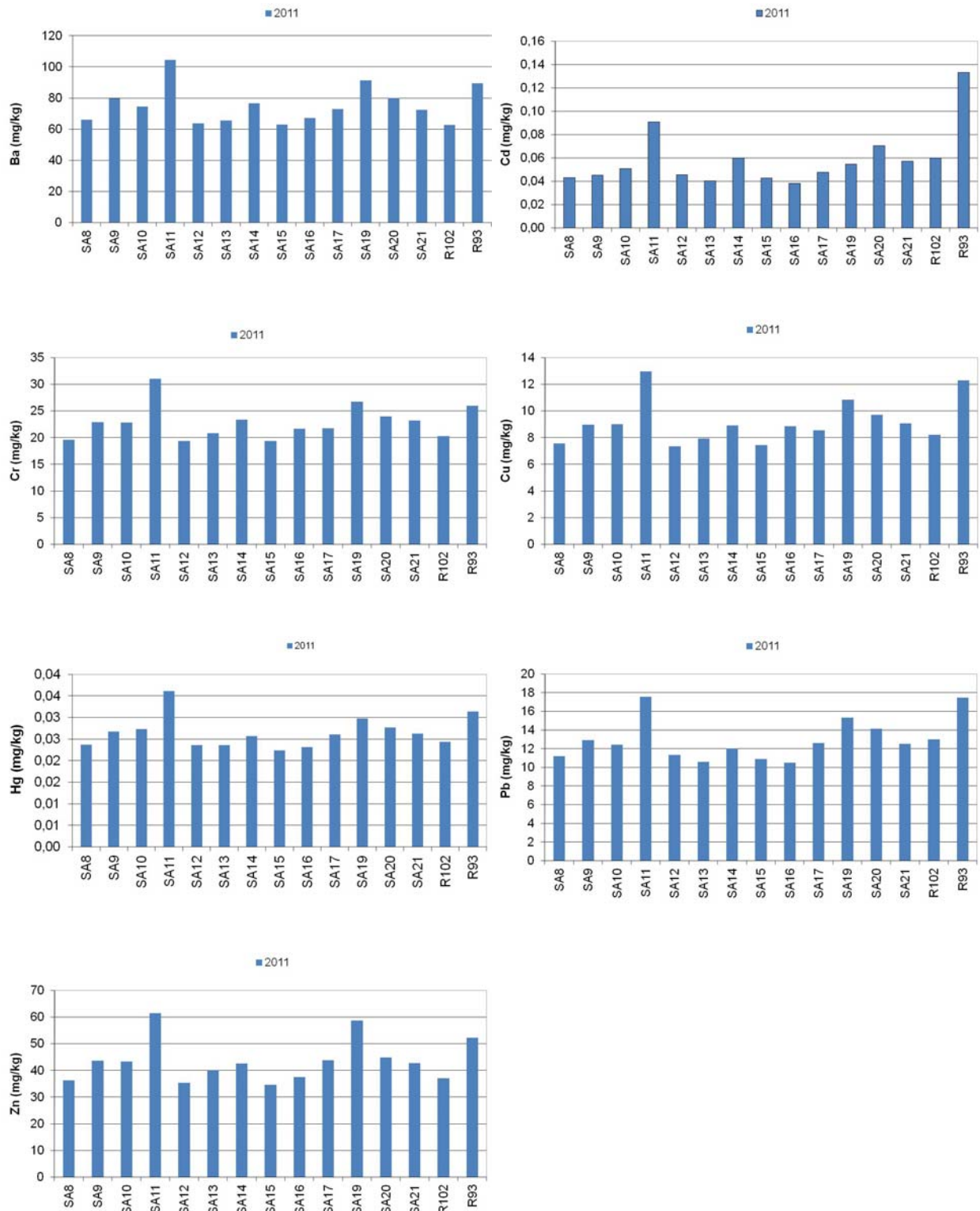
Figure 4.1-3 Salina 2011, the average content of metals in top sediment (0-1 cm) from three parallel samples.
